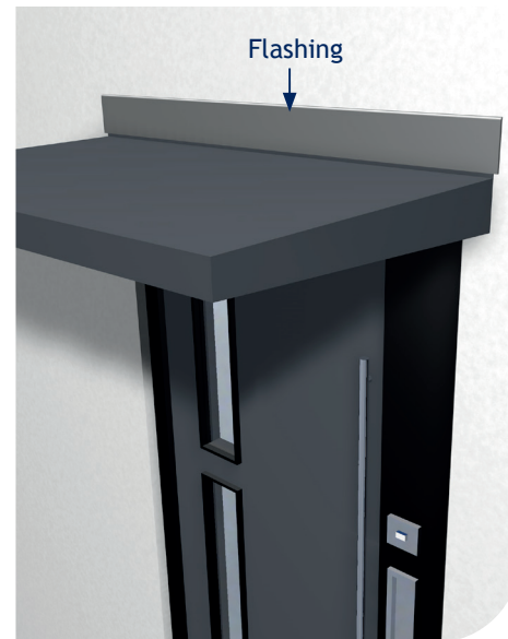
8. Finally, dress the top of canopy with lead or required flashing.
